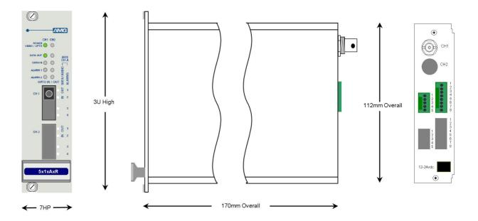
The **AMG5716A8R** is a rackmount one channel video receive unit designed to receive 1 video signal plus 6 Uni-directional alarms and transmit and receive 1 data signal over one Singlemode optical fibre.
